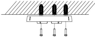
Figure 2-3 Attach the Mounting Base to the Ceiling
